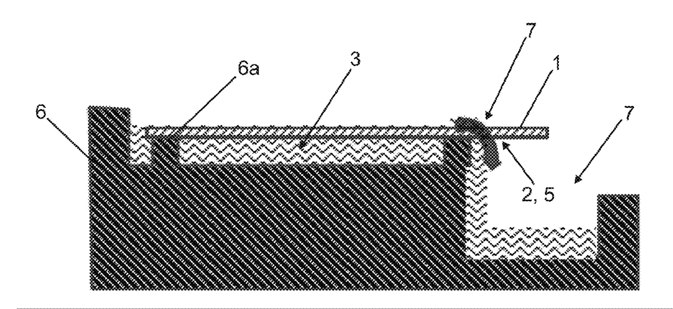
casting compound in the casting mold, wherein the translucent carrier and the casting compound (3) together form an optical system (10).
