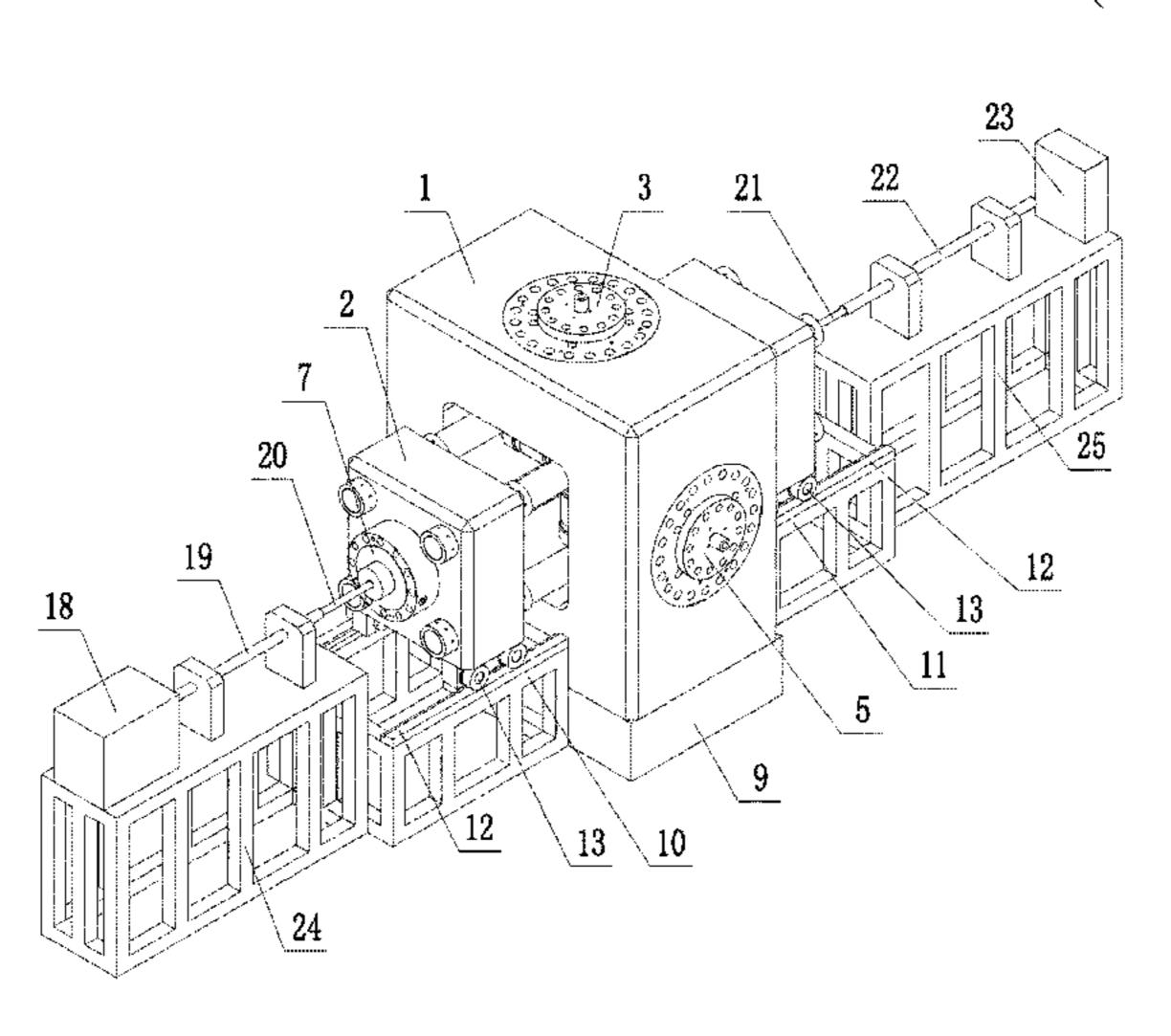
and the dynamic loading actuators adopt a static pressure oilway balance support sealing manner and are connected with the hydraulic station system, each oilway is provided with an energy accumulator, and flow is increased by the servo valves to drive pistons to perform dynamic response.
