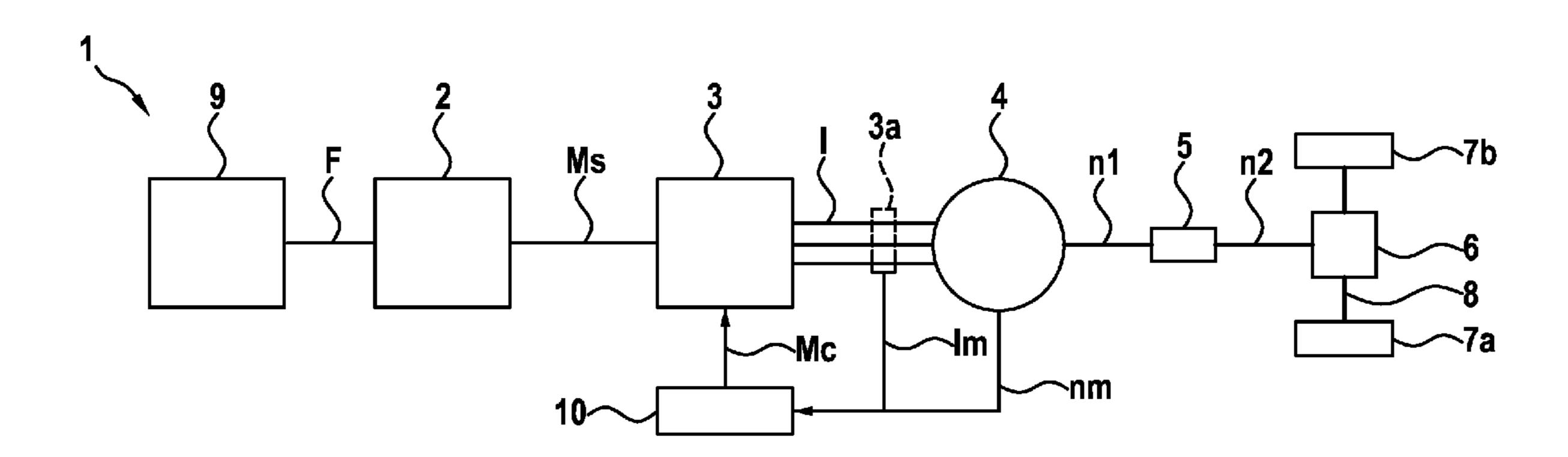
the determined present rotational speed, and a slip control unit, which is coupled to the computing unit and which is designed to at least temporarily apply a current correction amount to the output current of the voltage transformer if the present change of the wheel speed of the wheels exceeds a first predetermined threshold value.
