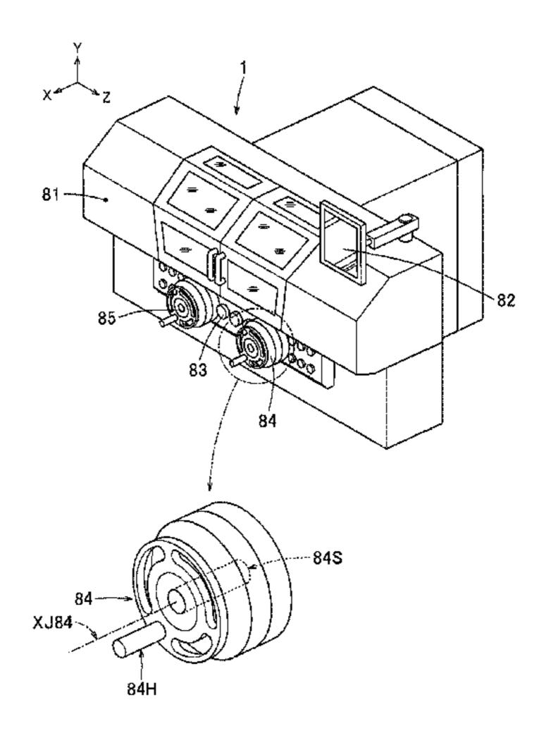
varying apparatus. The control apparatus controls the rotational-torque varying apparatus based on the proximity detection signal.
