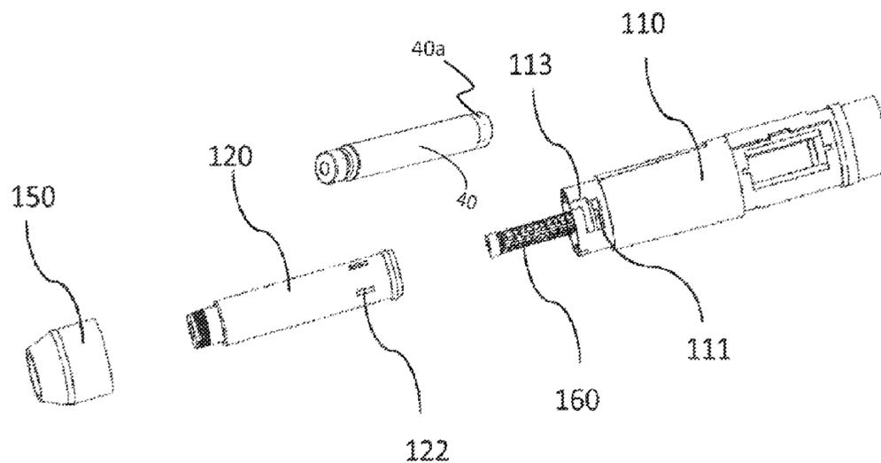
means arranged to match and interact with the third (**11**; **111**) and the fourth (**22**; **122**) mechanically coded interface means when the distal and the proximal housing parts are connected to each other.
