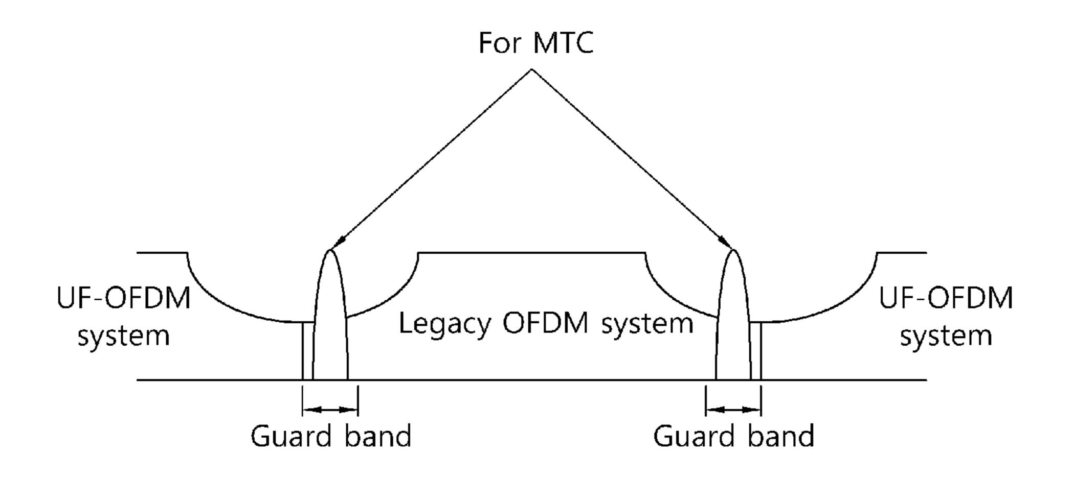
while performing frequency resource allocation between the first and second OFDM systems in accordance with the determined sizes of the frequency resources. The information regarding the frequency resource allocation, which comprises information indicative of either the guard carrier or the subcarrier, is transmitted.
