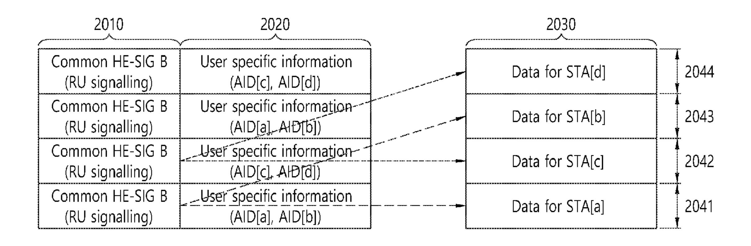
field corresponding to the particular frequency band can be used for scheduling of a data field corresponding to the same frequency band and a data field corresponding to another frequency band.
