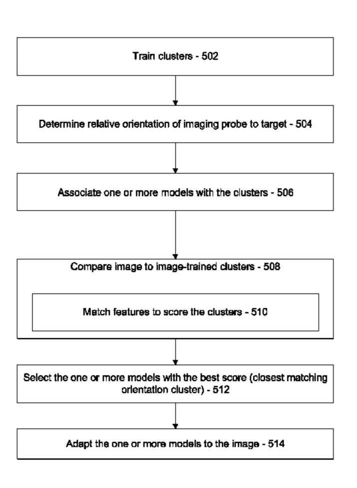
entation and is configured to select the one or more models based upon the cluster with the closest matching orientation. A model adaptation module (126) is configured to adapt the one or more models to the ultrasound image.
