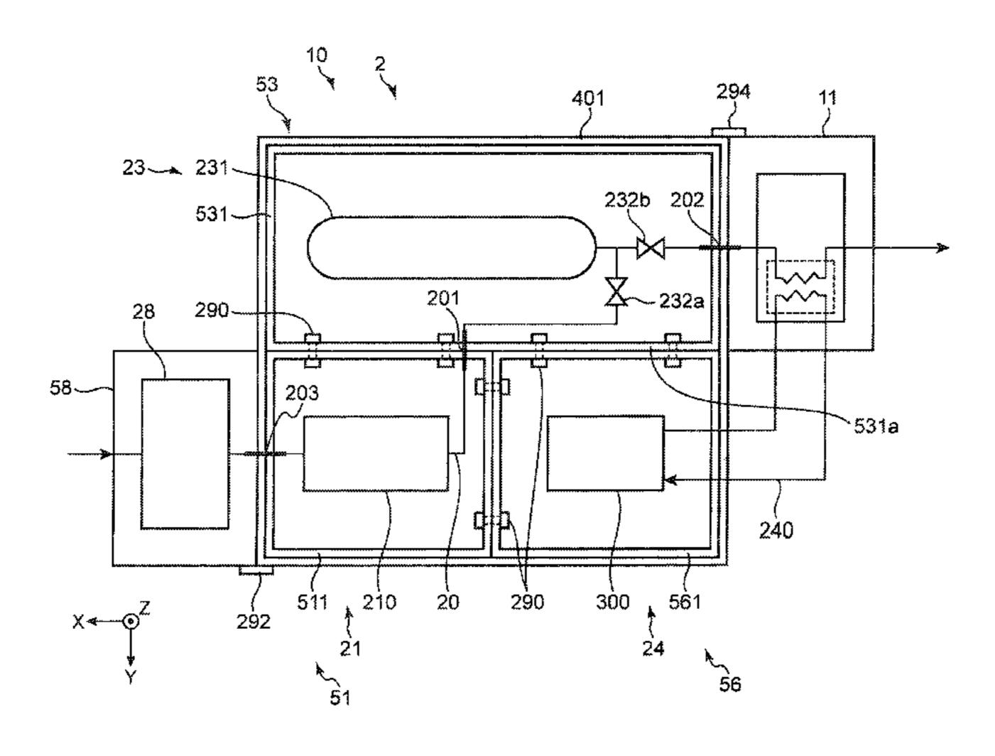
an expansion part, and a compression part; and a cooler accommodating body for accommodating the evaporation part, the expansion part, and the compression part. The compressor accommodating body and the cooler accommodating body are detachable from each other.
