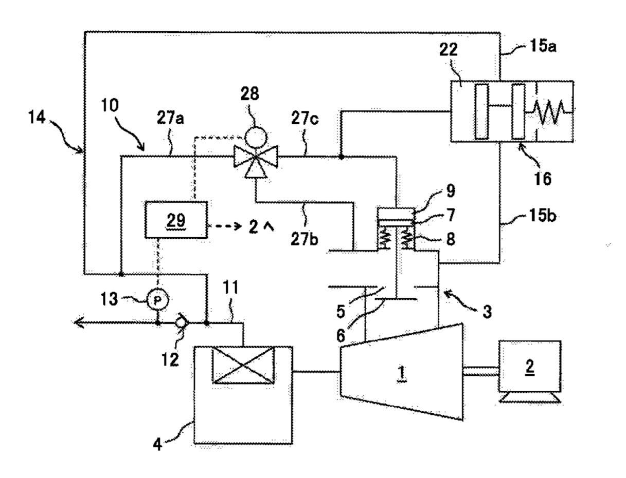
air-pressure operation circuit having a solenoid-operated three-way valve.
