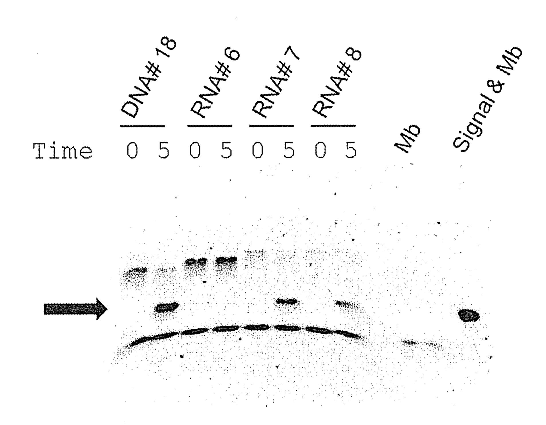
12% TBE-PAGE 180V, 45 min Loading Vol. 15 uL (+ 3 uL 6 × Dye)
