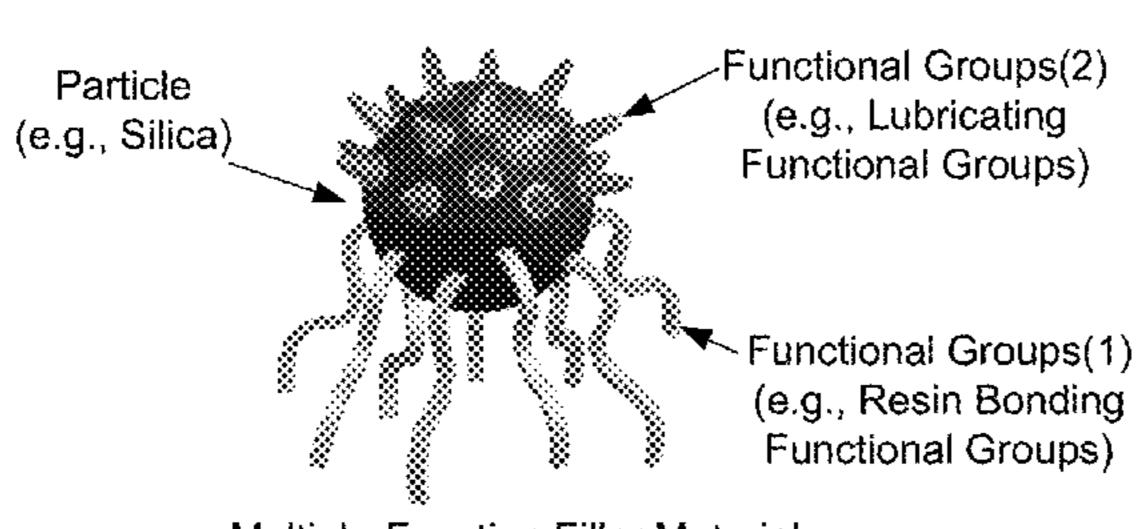
Multiple-Function Filler Material (for polymeric applications)
