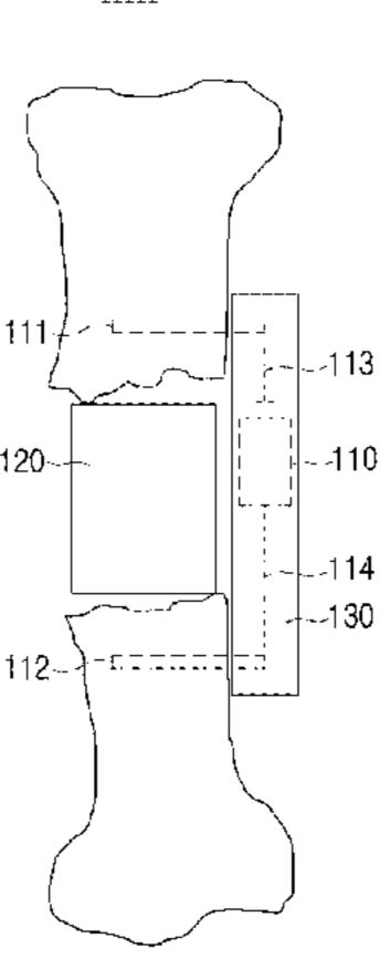
a first electric conductor to be connected to a first electrode of the battery and inserted into a bone located on one side of the scaffold; and a second electric conductor to be connected to a second electrode of the battery and inserted into a bone located on the other side of the scaffold, wherein the battery forms an electric field on the scaffold by applying voltage to the first electric conductor and the second electric conductor.
