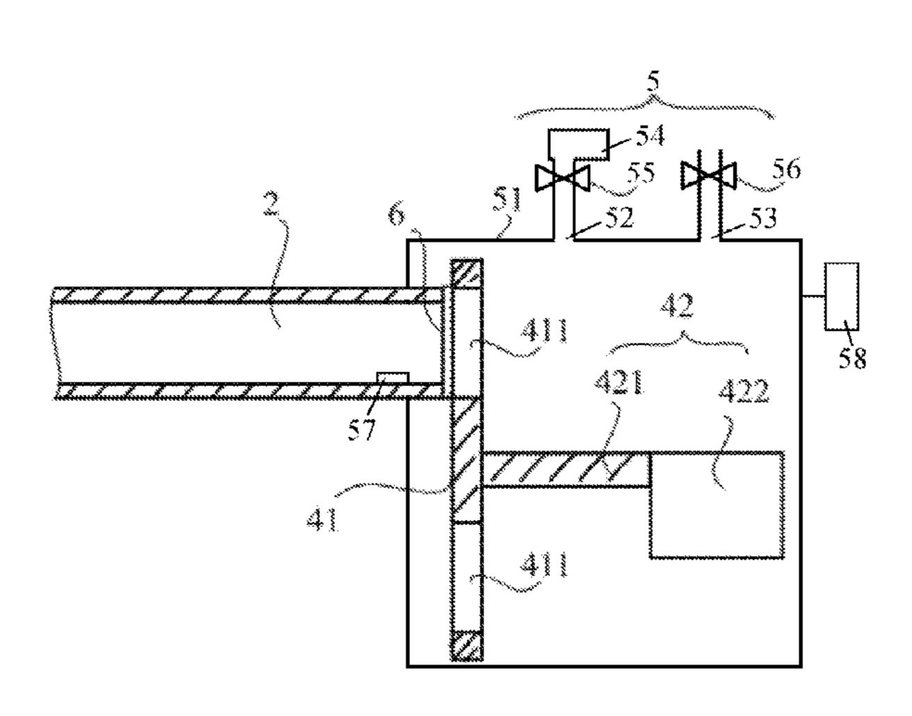
The support plate is provided with a plurality of windows, and the driving component is adapted for driving the support plate so that one of the plurality of windows seals a corresponding opening.
