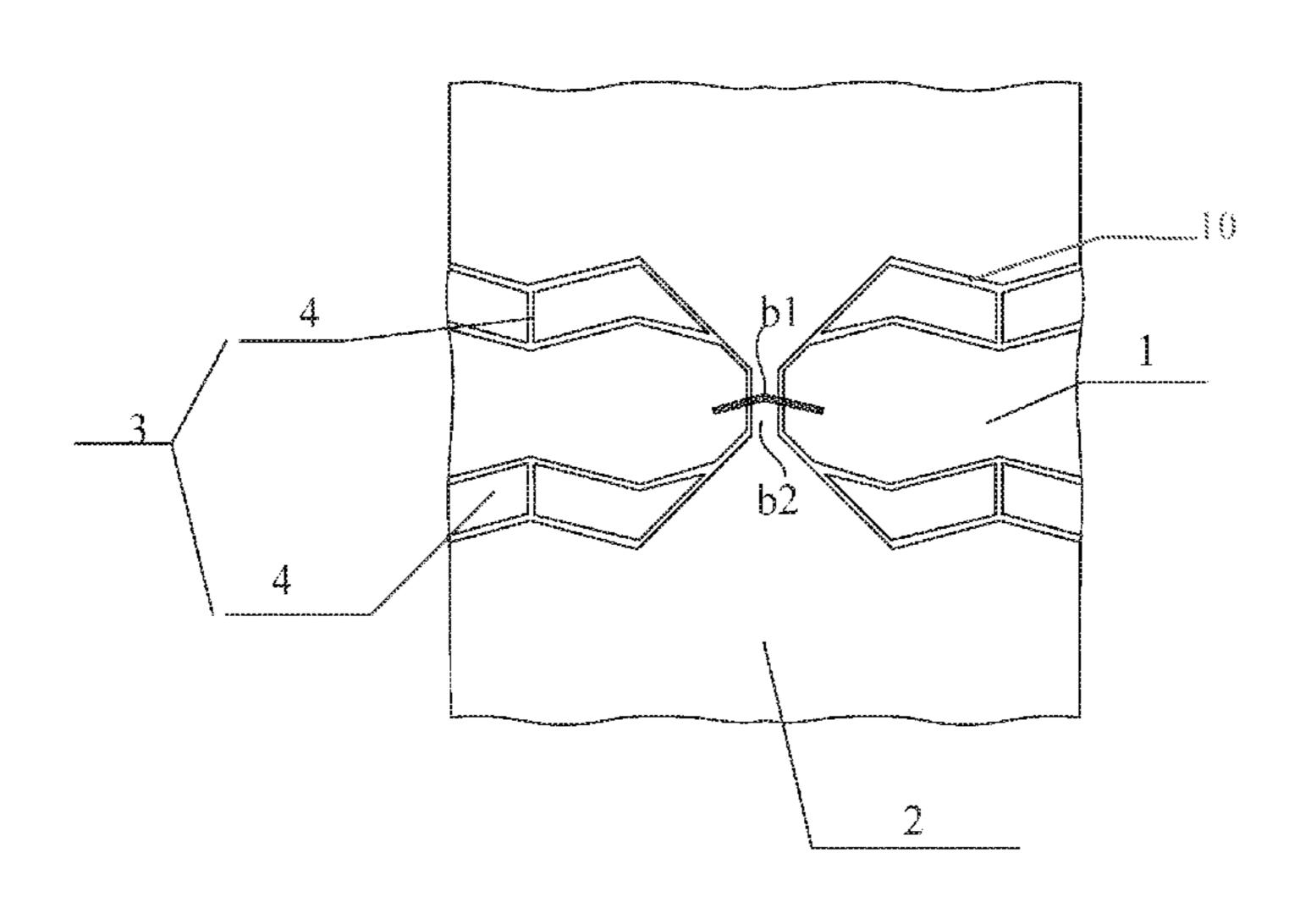
the second undulating boundary. The first electrode, the second electrode, and the fill pattern in a same electrode unit are electrically isolated from each other.
