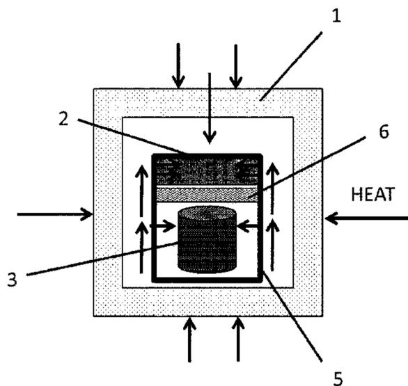
mally conductive materials can be referred to as conductive equalizers. The conductive equalizers can conductively transfer heat from the hotter portions of the interior of the container to cooler portions of the interior of the container and/or from portions of the interior desired to be cooled to the cold bank. Conducting heat from hotter portions to cooler portions, or from portions to be cooled to the cold bank can result in a more uniform temperature distribution around the product.
