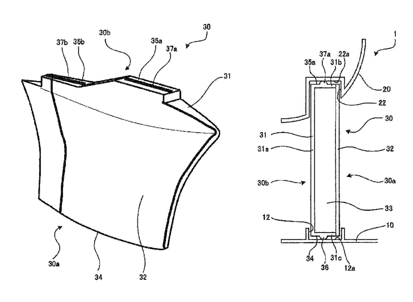
respectively directed onto and moved along the projection 36 and the projections 37a and 37b.
