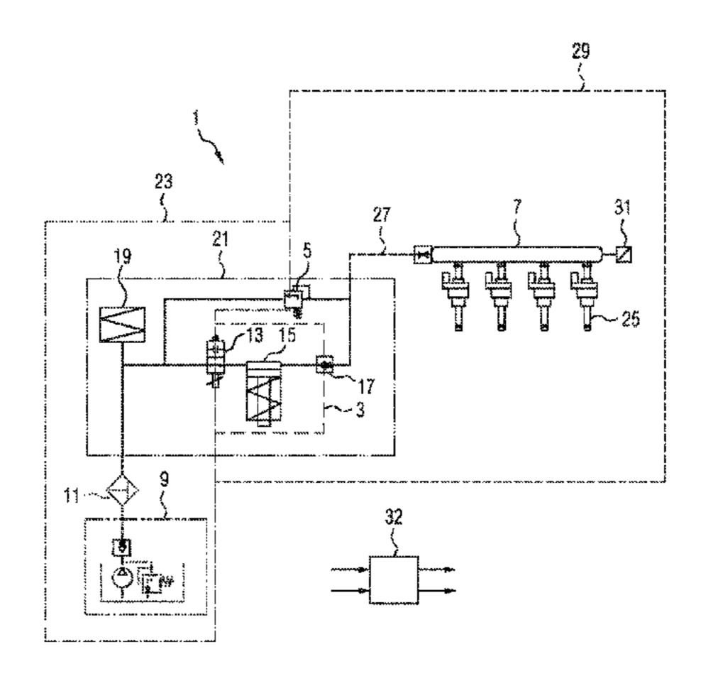
actuating the high-pressure pump such that, at the outlet side of the high-pressure pump, a pressure is increased such that the pressure-limiting valve is opened.
