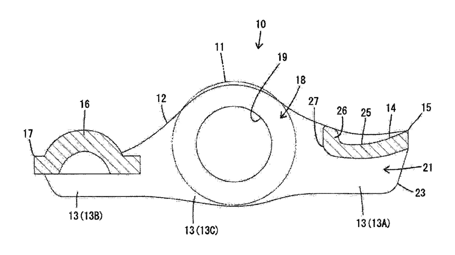
(14) so as to be opposed to each other and disposed along and in proximity to a side peripheral surface of the stem end (81A) of the valve (80). At least protruding distal ends of the sidewalls (13) each have a smaller thickness than adjacent portions and serve as a thinner portion (23).
