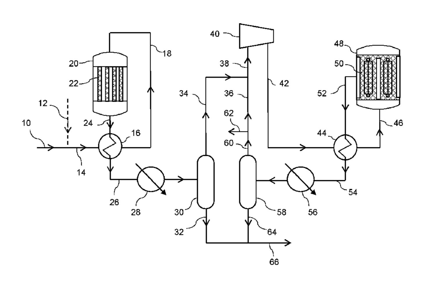
gas stream, wherein the first synthesis reactor has a higher heat transfer per cubic meter of catalyst than the second synthesis reactor, none of the loop recycle gas stream is fed to the first synthesis gas mixture and the recycle ratio of the loop recycle gas stream to form the second synthesis gas mixture is in the range 1.1:1 to 6:1.
