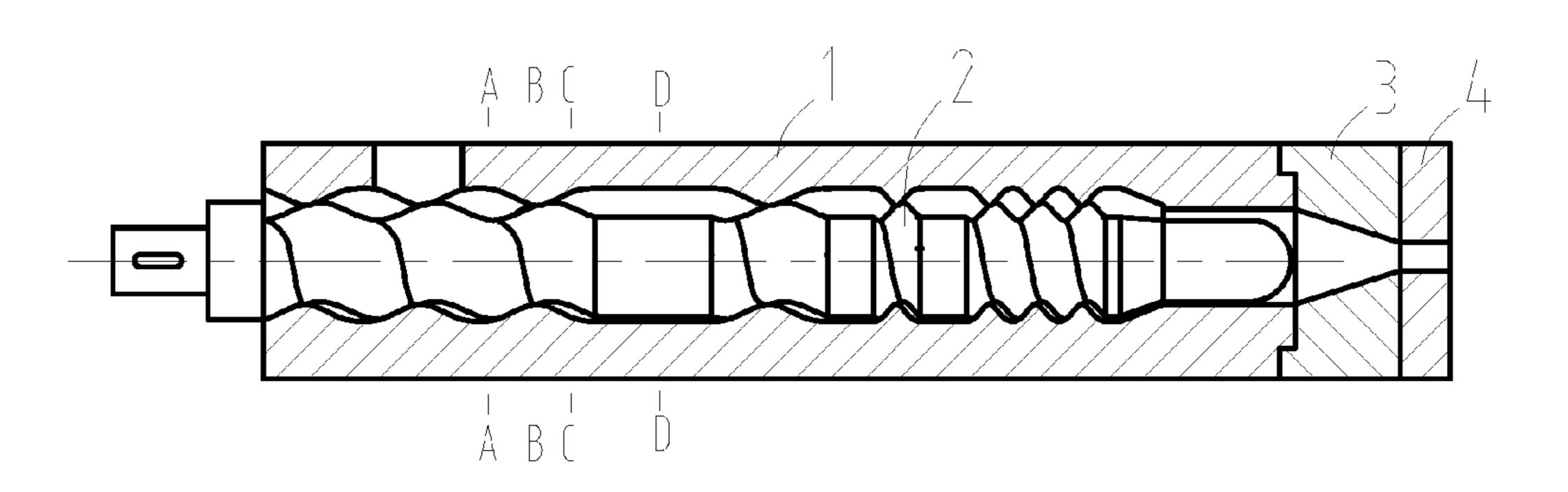
ments and the eccentric straight segments of the eccentric rotor correspond one-to-one with the spiral segments and straight segments of the stator. The present invention can be used as the extruding system of an extruder or be combined with different plunger injection units to form a plasticating injection device of an injection molding machine. The present invention has a short thermo-mechanical distance for the materials, low energy consumption, and wide adaptability.
