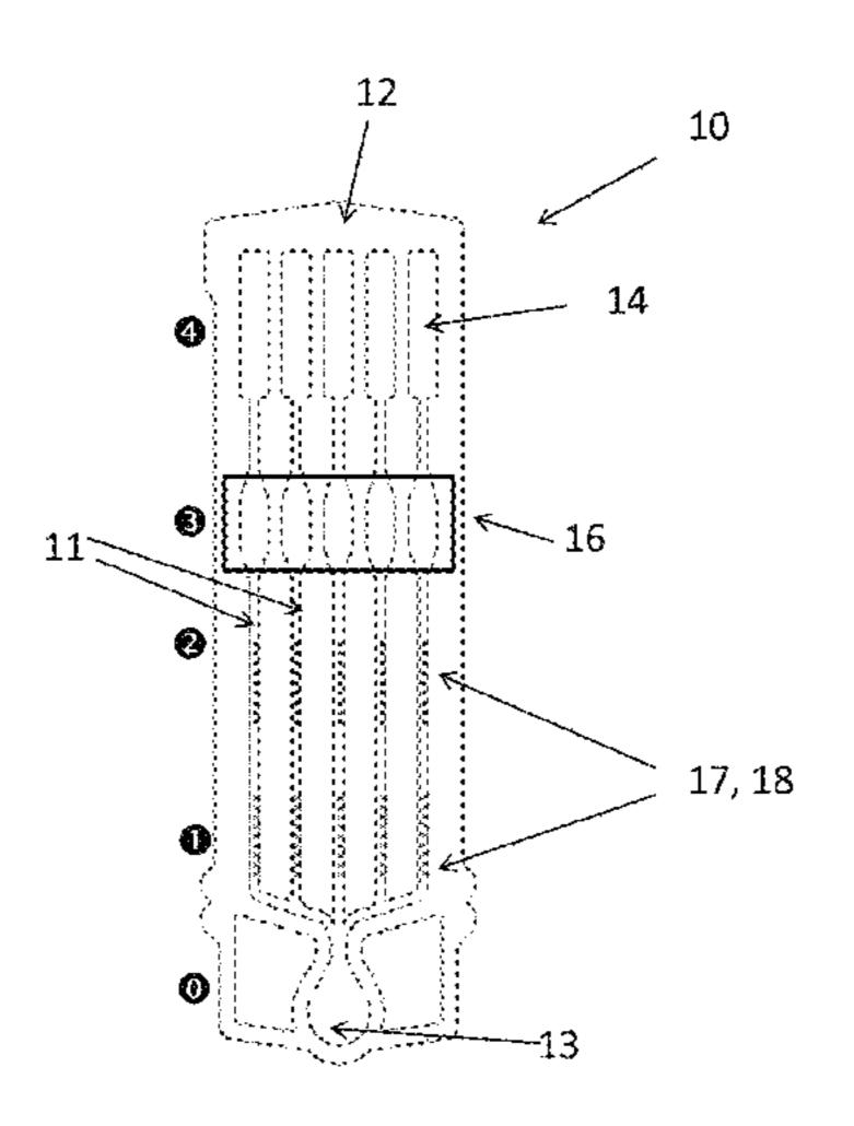
the first optical detection sites of the microfluidic cartridge is positioned in the beam path of the first light source, and when the cartridge is inserted to a second predetermined position into the slot, another one of the first optical detection sites of the microfluidic cartridge is positioned in the beam path of the first light source.
