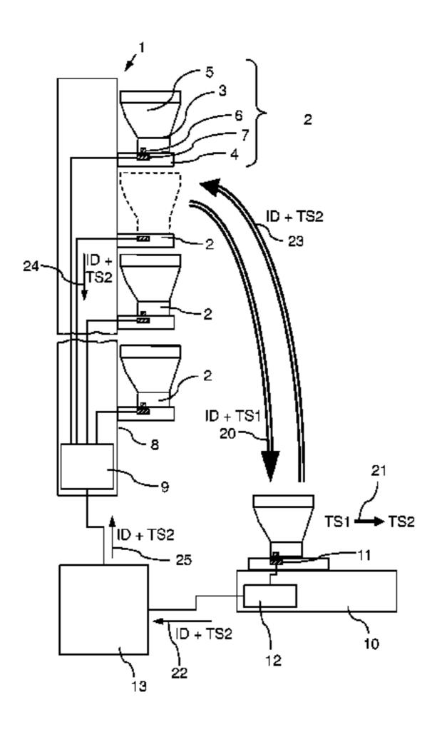
memory location for a filling code. Every time the reservoir has been refilled, the filling code is changed at the charging station so that the refilling can be detected by the control device when the information memory is read by the reading device after the removable part has been placed back onto the stationary part of the same or a different storing and metering station.
