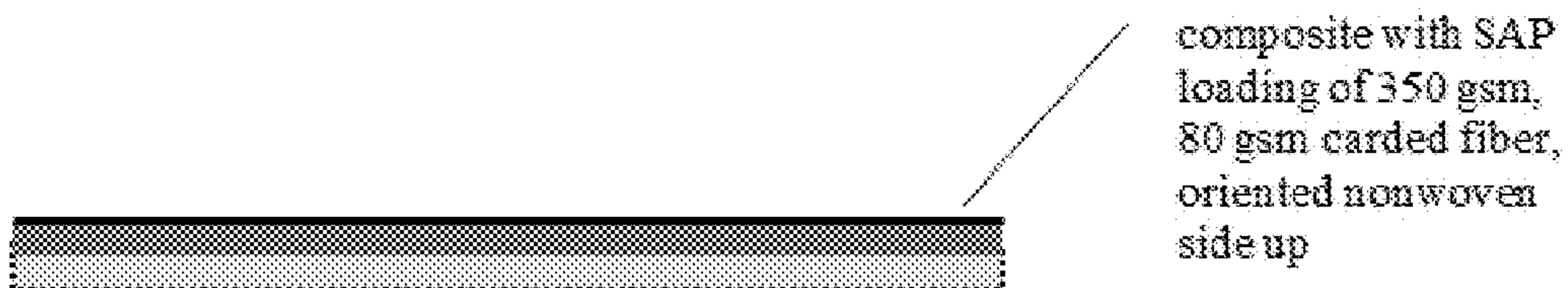
Figure 13: Core C – cross-section view (high SAP loading, high basis weight carded fiber)
