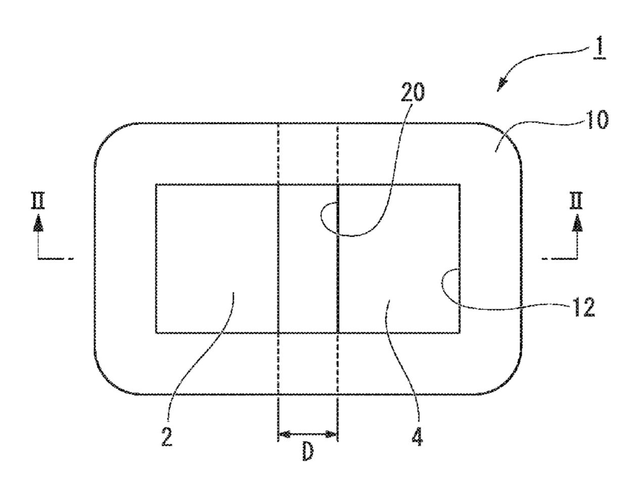
tive adhesive sheet has a thickness compressibility of 10% or less and a thickness recovery ratio of 95% or more. The base is a non-electroconductive base having a water absorption capacity of 1 to 1.5 times, and the pad has a moisture permeability of 1,000 g/m²/24 h or more.
