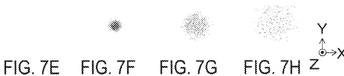
© IRRADIATION SPOT SIZE OF MAIN PULSE LASER BEAM
