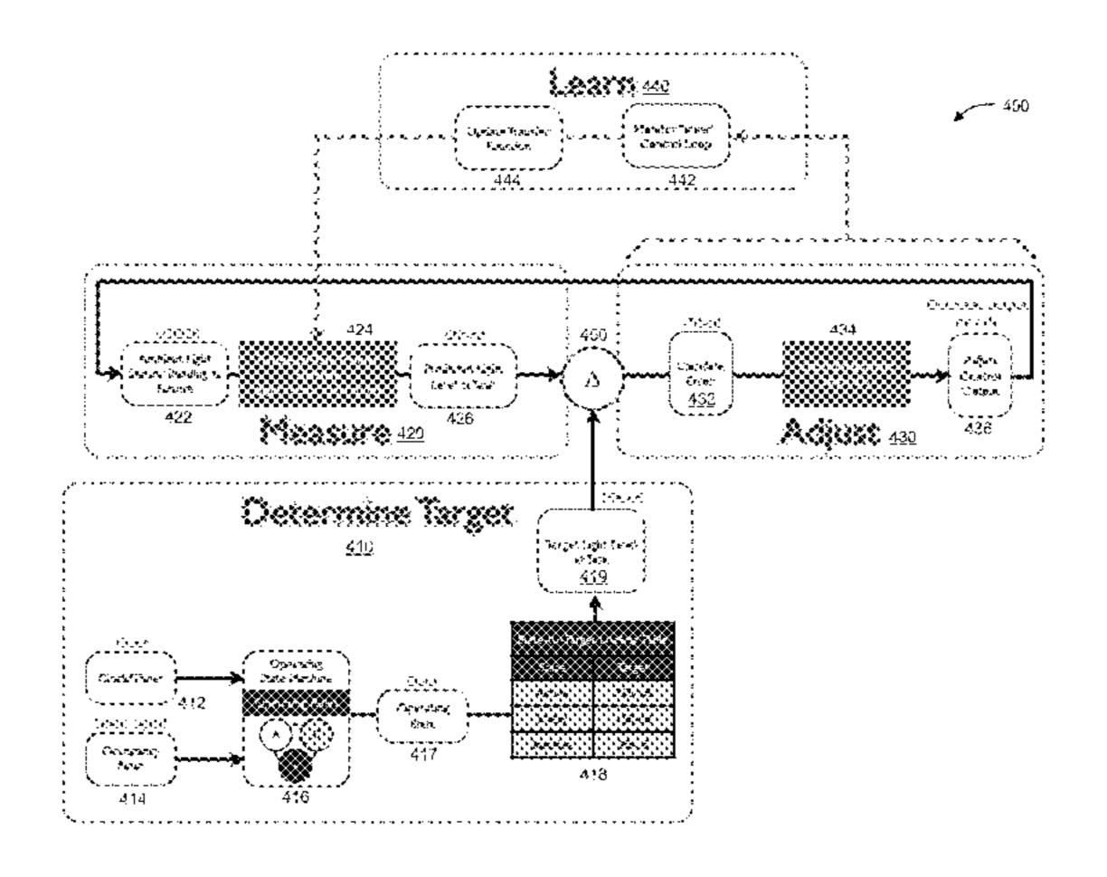
determine the difference between the estimated ambient light level and a desired light level at the task height, and may change the artificial illumination provided by a light fixture to make the actual ambient light level at task height match the desired light level at the task height.
