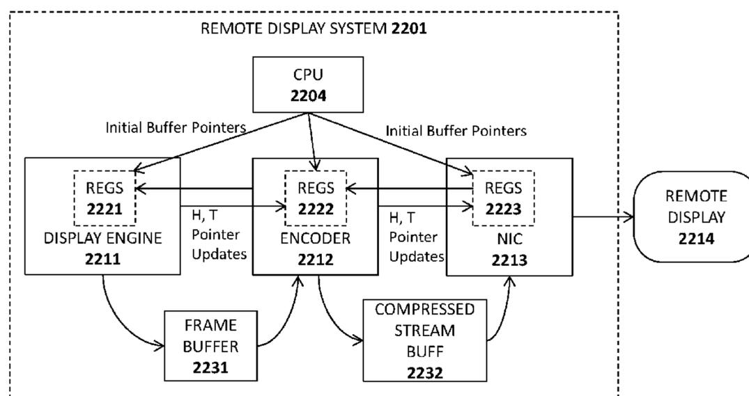
updated without intervention from the CPU as the display engine writes to the frame buffer, the encoder reads from the frame buffer and writes to the compressed stream buffer, and the network interface controller reads from the compressed stream buffer.
