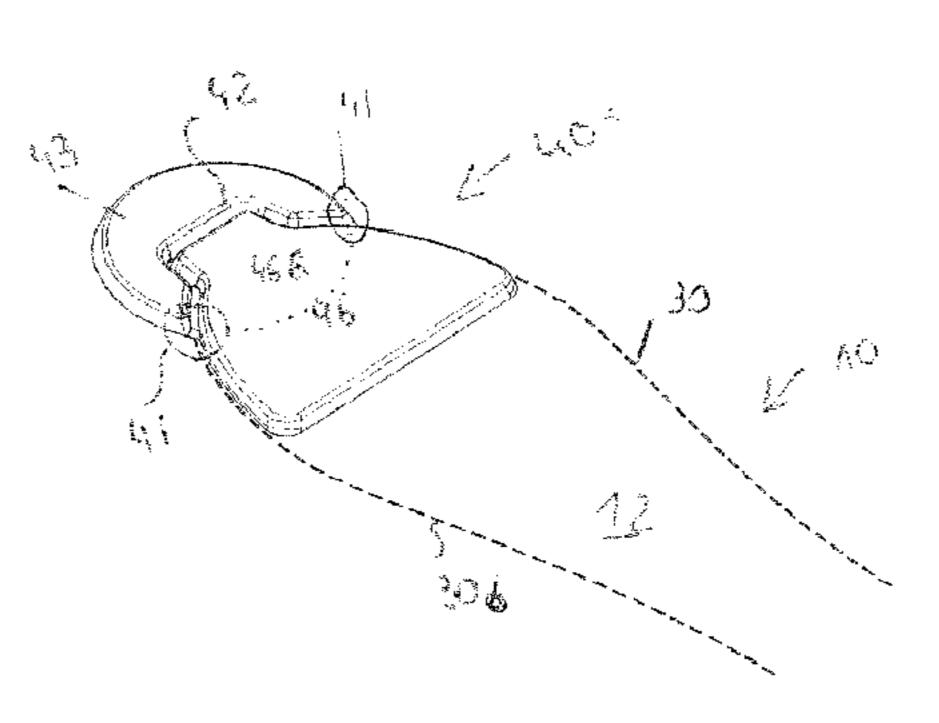
adjacent and to the weakening lines (30, 30b) as to facilitate rupturing substantially along the at least one weakening line.
