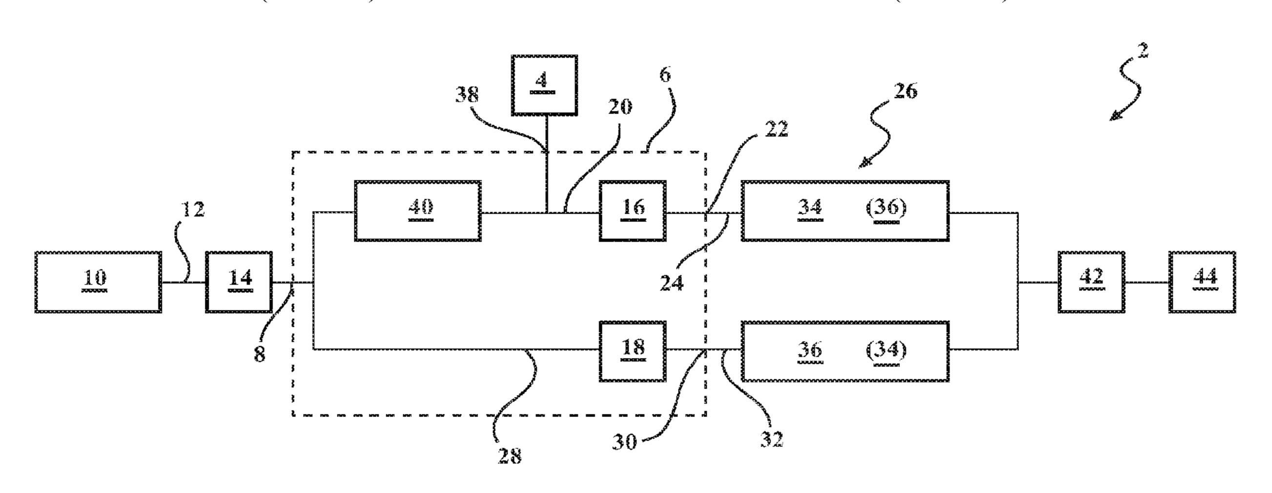
which interacts with the electric machine, and the second clutch arrangement has a second clutch input side, wherein the first clutch input side of the first clutch arrangement is connected to the input side of the double clutch device via a freewheel or to the second clutch input side of the second clutch arrangement.
