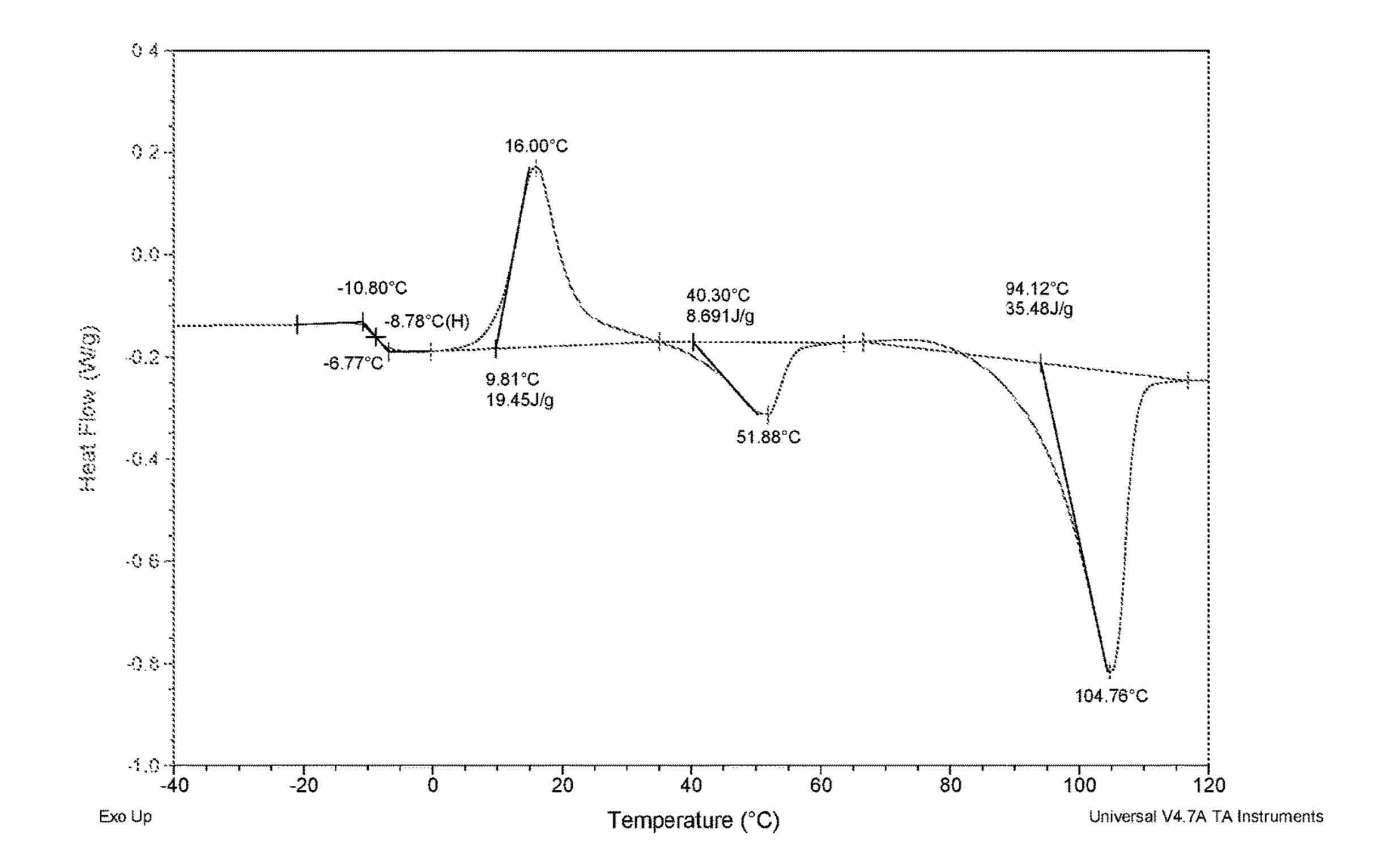
Figure 2. DSC Scan of the Second Heat Measurements for Inventive Monofilament of Example 3B
