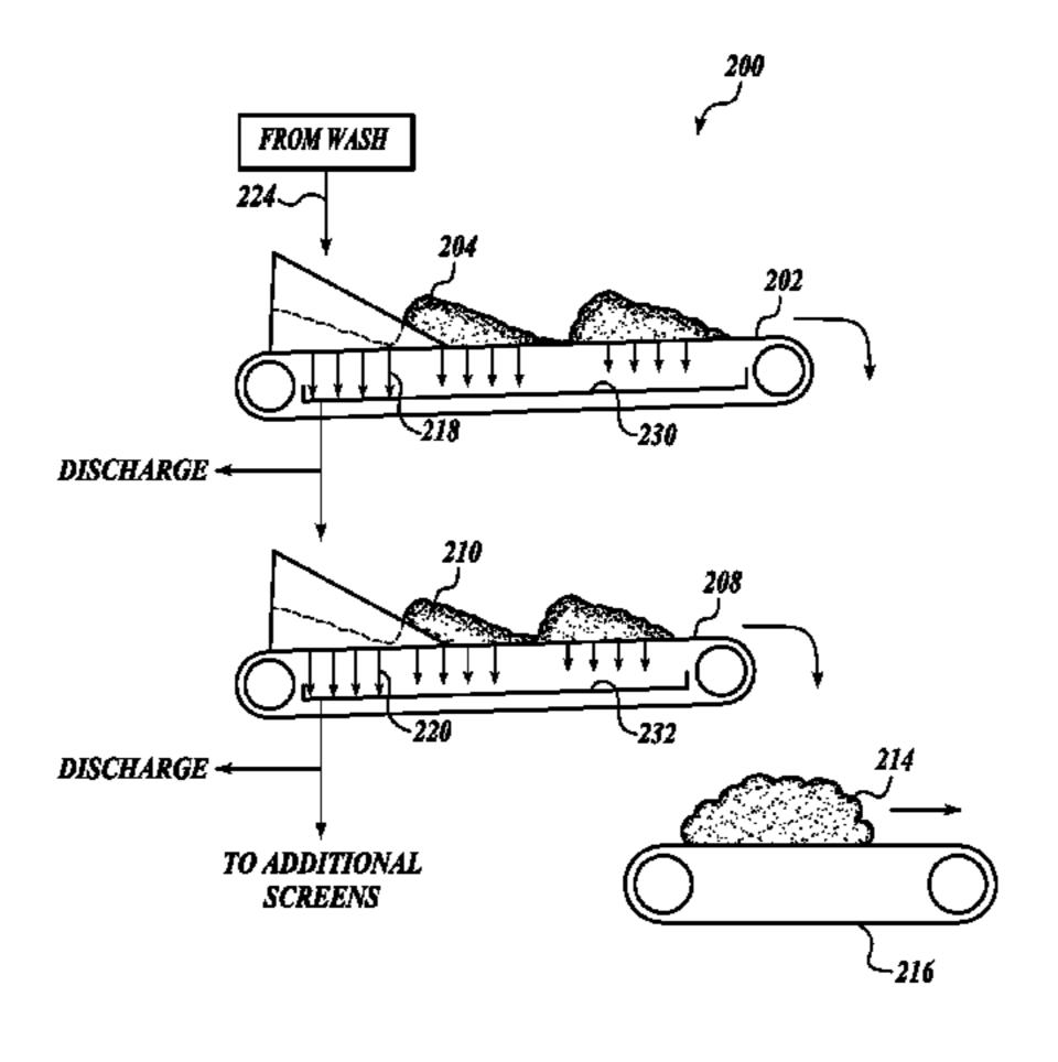
intermittently, while the wash water is allowed to percolate through the fish flesh and exit the perforated screen.
