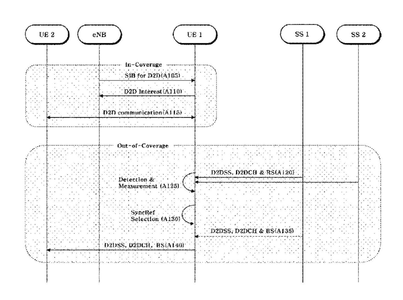
from said at least one synchronization source according to whether a prescribed condition is satisfied, wherein said prescribed condition is satisfied if the measured result of the D2D reference signal satisfies a threshold value and an information element of a D2D channel linked with the D2D reference signal satisfying the threshold value is acquired.
