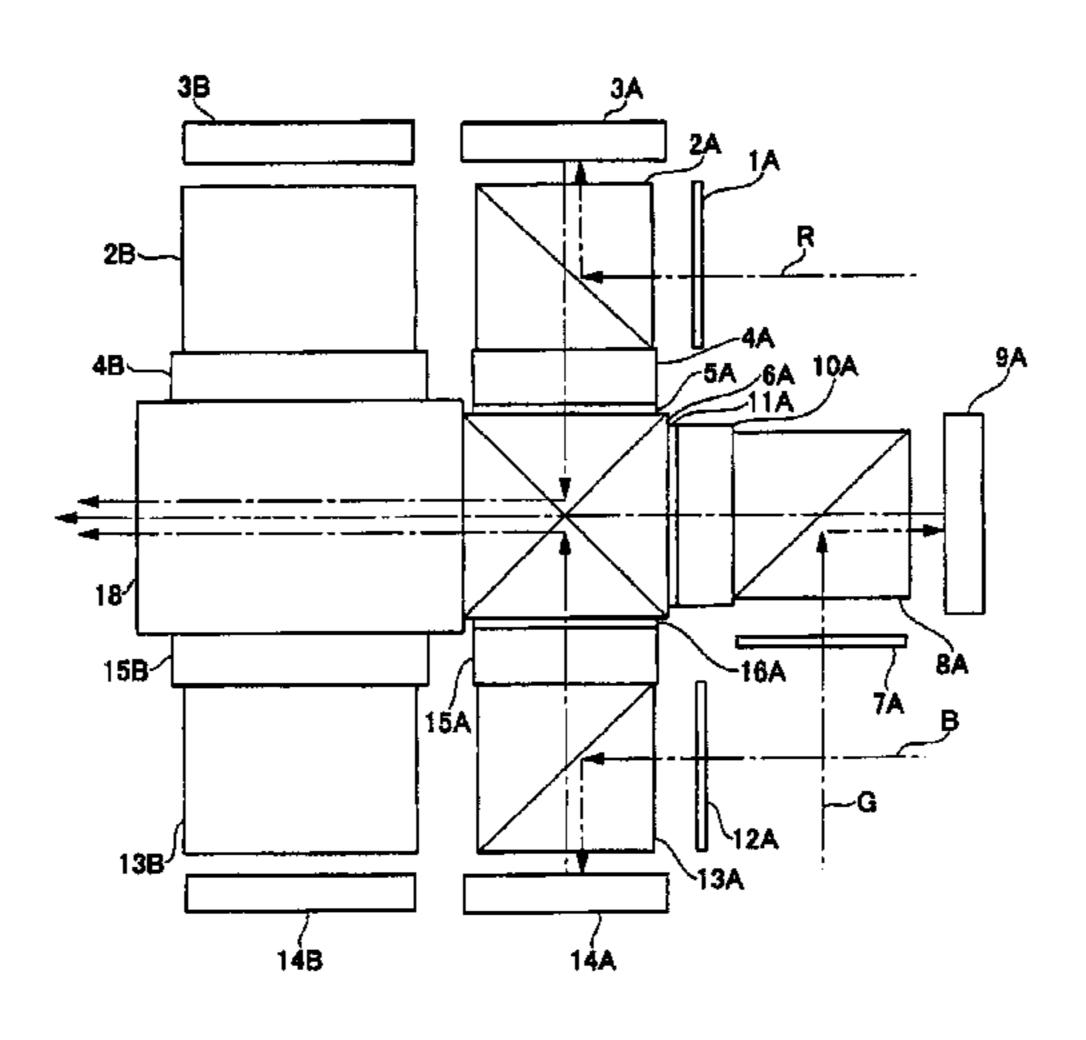
a second prism-type photosynthesizing member having a function of synthesizing, on one optical axis, light that is reflected by the second reflection-type light valve group; and a prism-type beam splitter configured to synthesize, on one optical axis, light that has been reflected by the first reflection-type light valve group and light that has been reflected by the second reflection-type light valve group.
