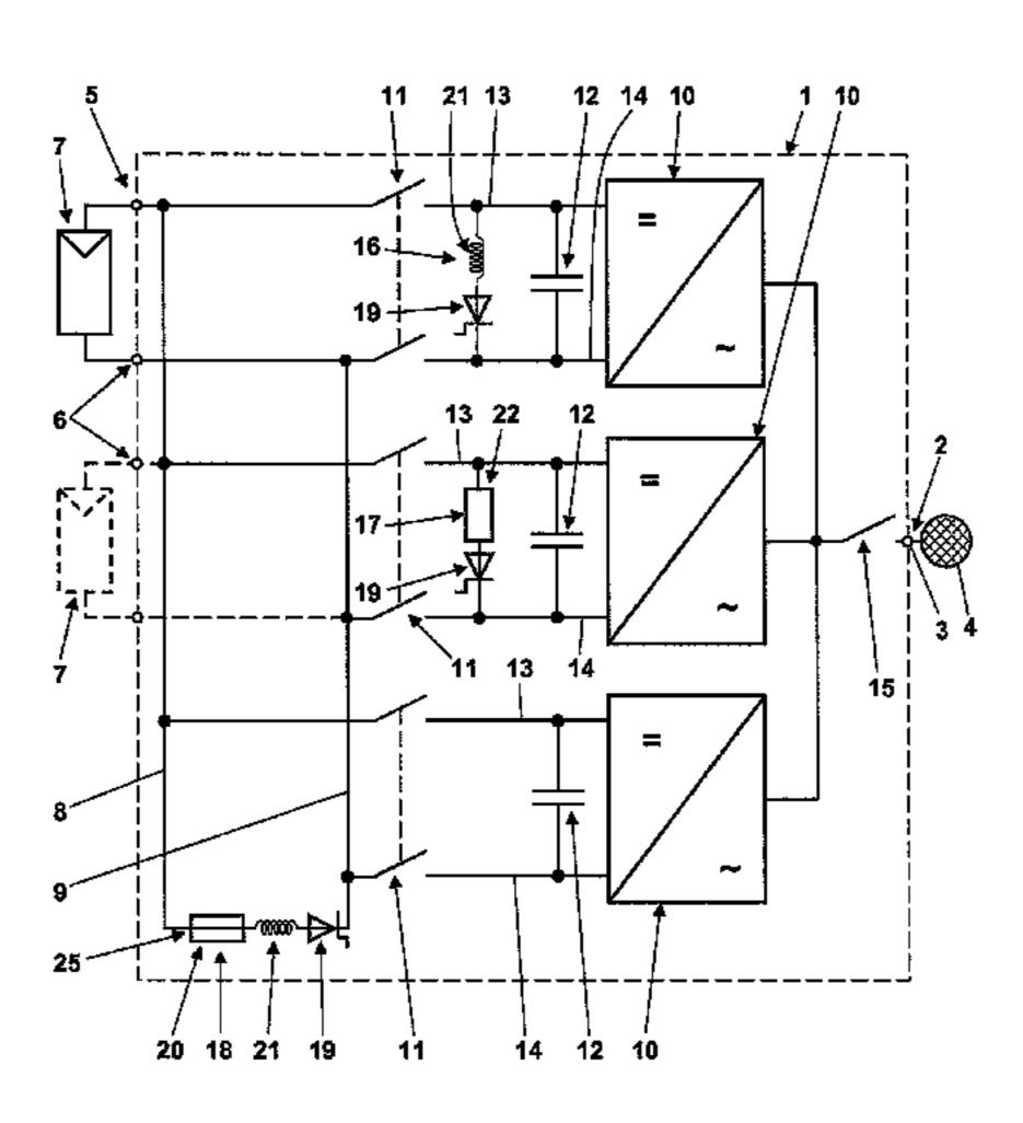
one short-circuit path between the bus lines is connected in series with a fuse. Still further, the circuit arrangement includes at least one further short-circuit path for short-circuiting the voltage between the bus lines, wherein a short-circuit switch likewise is arranged in the at least one further short-circuit path.
