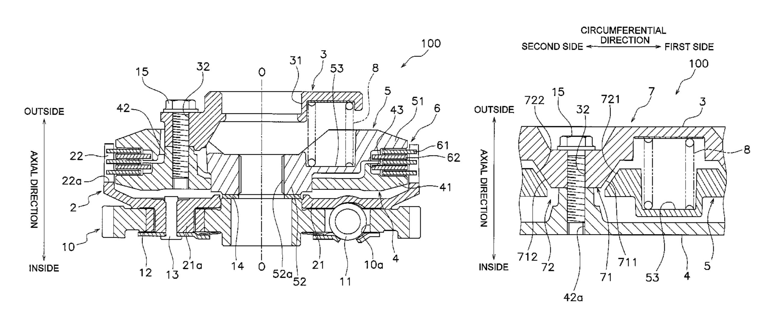
tilt to face axially inside and face oppositely to each other in a circumferential direction. The third cam surface is opposed to the first cam surface. The fourth cam surface is opposed to the second cam surface.
