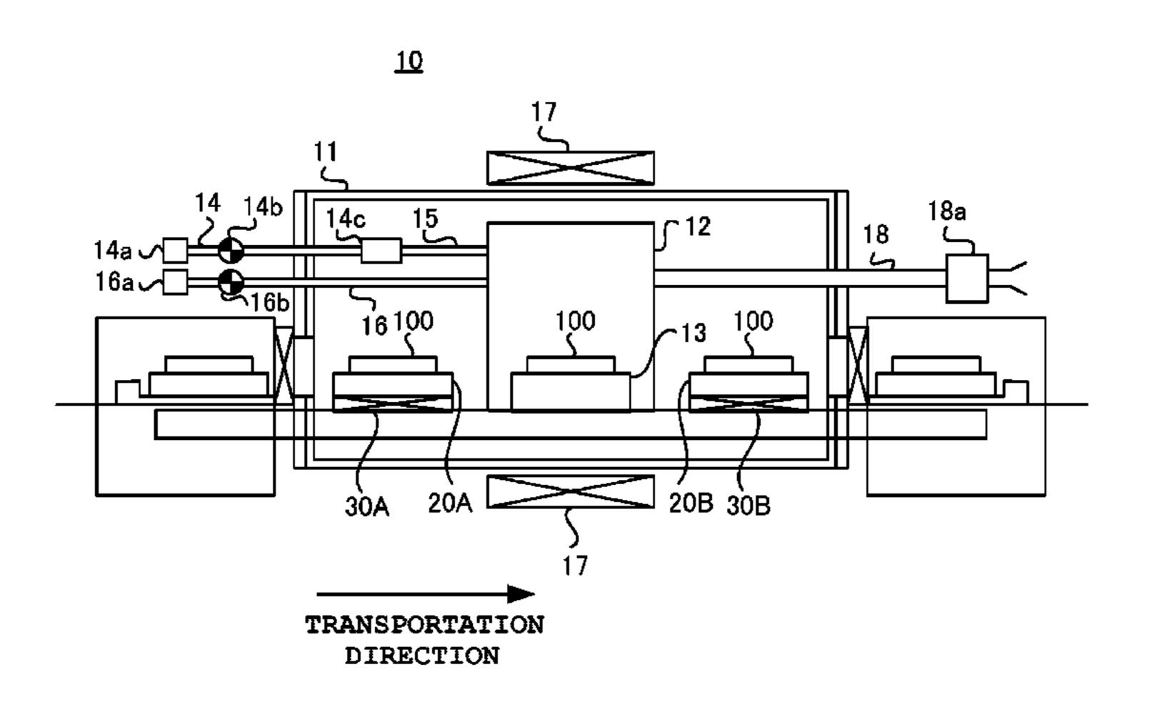
table so that the temperature of the processed substrate unloaded from the processing part is lowered to a predetermined temperature, before the substrate is placed on the substrate placing table, when the substrate placing table is provided to the temperature lowering part.
