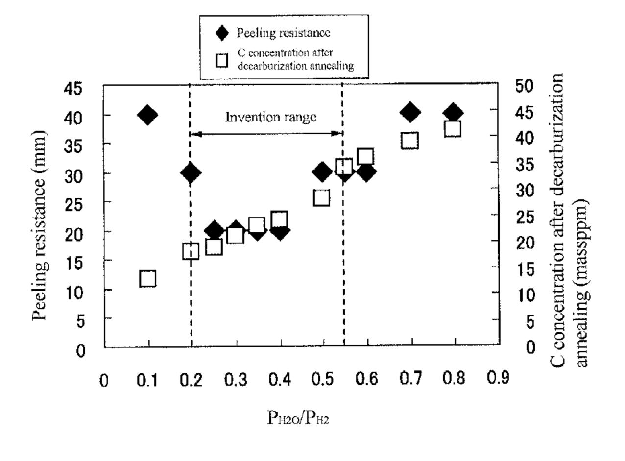
C./s and heating rate R2 between T1 and T2 is set to not more than 15° C./s, whereby grain-oriented electrical steel sheet having excellent iron loss property and coating peeling resistance is obtained in the inhibitor-less ingredient system while ensuring decarburization property even when rapid heating is performed during decarburization annealing.
