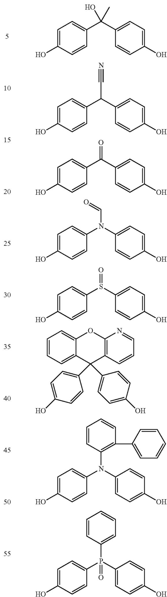
Dihydric phenol compounds of Formula (III) can be converted to a diepoxide using any suitable process and materials. The use of epichlorohydrin in the epoxidation process is presently preferred. By way of example, below is a diepoxide formed via an epichlorohydrin epoxidation of 4,4'-methylenebis(2,6-di-t-butylphenol).
