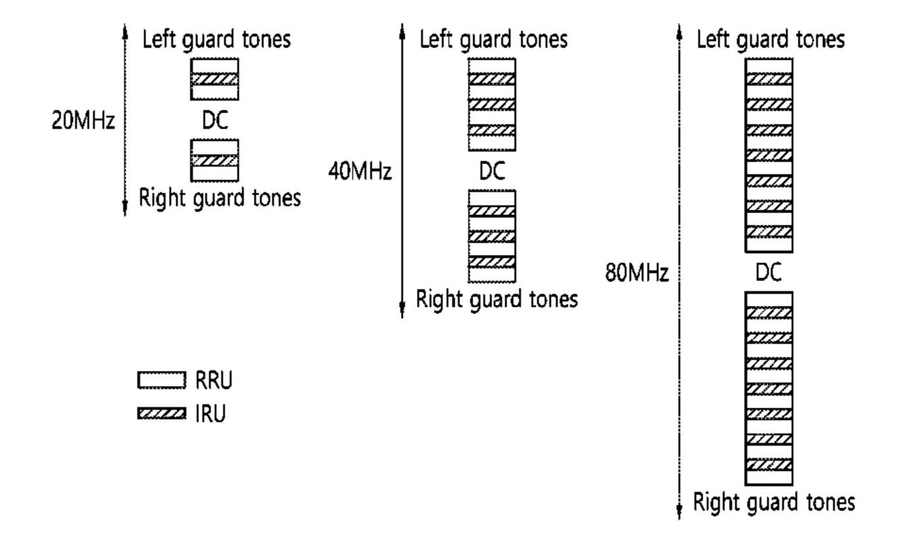
each of the plurality of wireless resources can be a combination of a plurality of wireless resource units defined as having different sizes from each other on a frequency axis.
