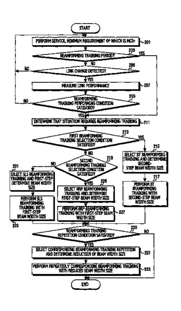
a channel link between the network node and another network node; identifying a beamforming training scheme based on the at least one factor value; and performing beamforming training with the another network node by means of the selected beamforming training method, thereby finding an optimal beam for maintaining services through the most efficient method according to a channel state and minimizing the time consumed for beamforming training.
