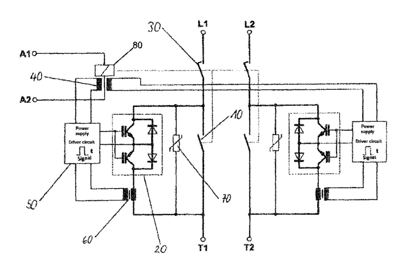
designed to switch the semiconductor switch on and off and which are supplied by the voltage produced in the auxiliary coil when the voltage supply of the switching drive is switched off.
