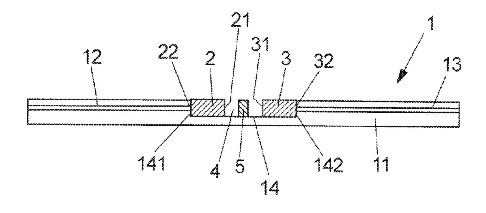
and the first and the second reflective structure are at least partly arranged in a cutout of the substrate or adjoin the cutout.
