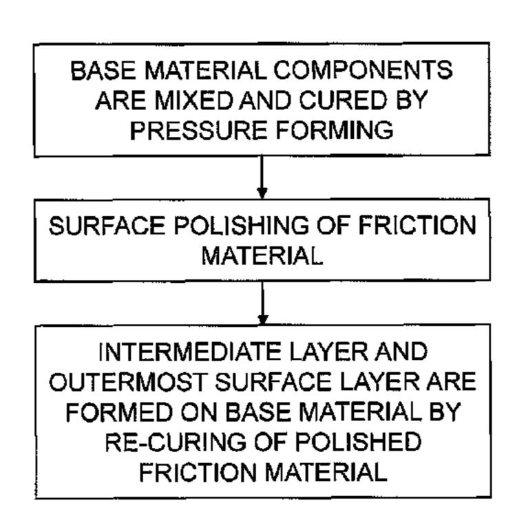
on the base material. The intermediate layer includes either a glassy carbon structure or a graphite structure formed as a result of thermal curing of the thermosetting resin contained in the base material. In addition, the clutch friction material includes an outermost surface layer disposed on the intermediate layer. The outermost surface layer contains a pyrolysate produced as a result of pyrolysis of rubber and resin components contained in the base material.
