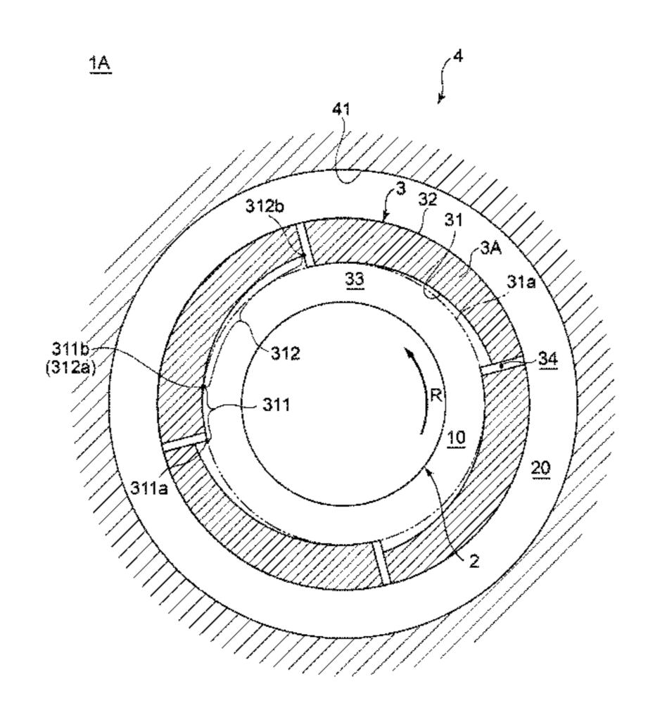
at a position recessed from the land portions, the recess portions being configured such that a distance between the recess portions and a virtual true circular line (31a, 32a, 41a) passing through the land portions increases in a direction opposite from a rotational direction of the rotational shaft (2) from end portions (311b, 321b, 411b) of the land portions opposite from the rotational direction of the rotational shaft.
