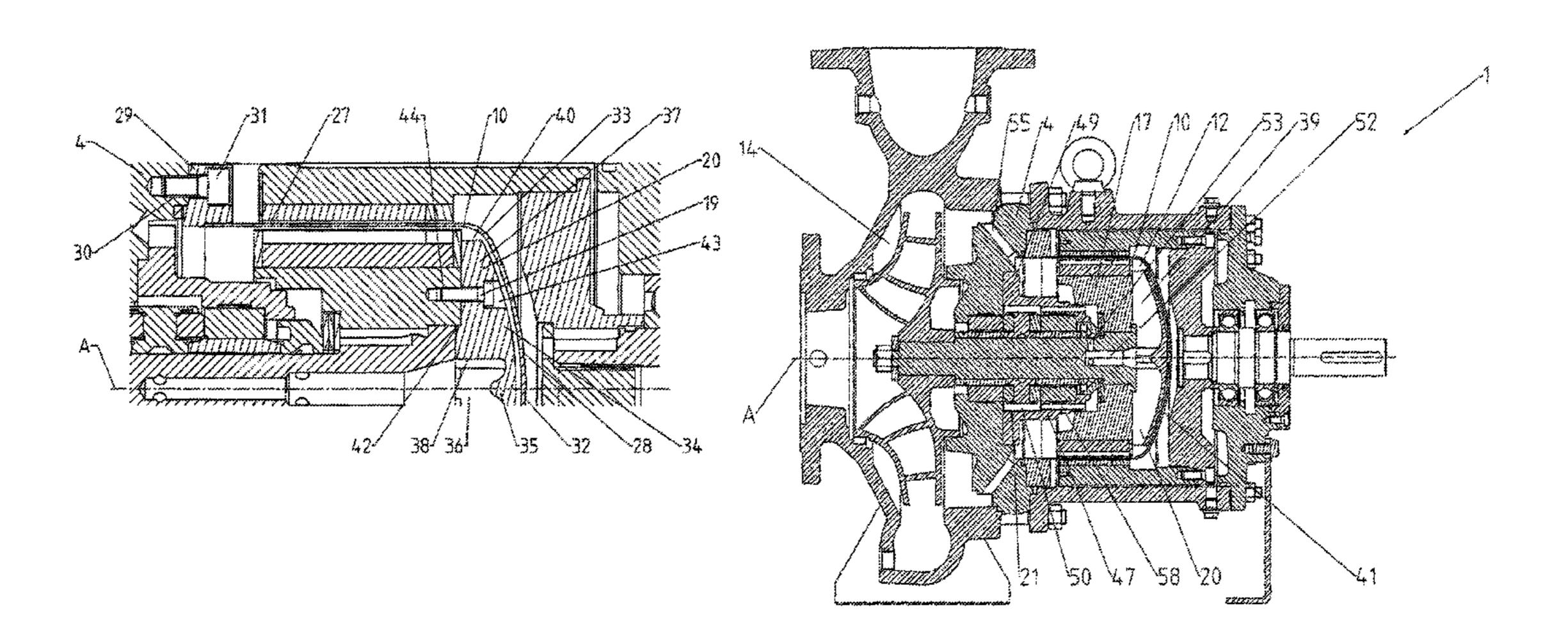
chamber adjacent to a domed base of the containment can. The auxiliary impeller is secured to the inner rotor and includes vanes and impeller channels for circulation of media.
