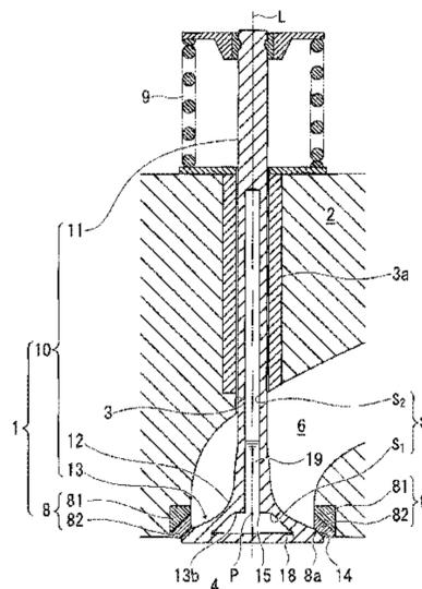
layer having thermal conductivity of 23-50 (W/m·K) at 20-300° C. and a valve contact face side layer having thermal conductivity of 10-22 (W/m·K) at 20-300° C. This enables a valve temperature decrease throughout an engine's entire RPM range compared with the prior art.
