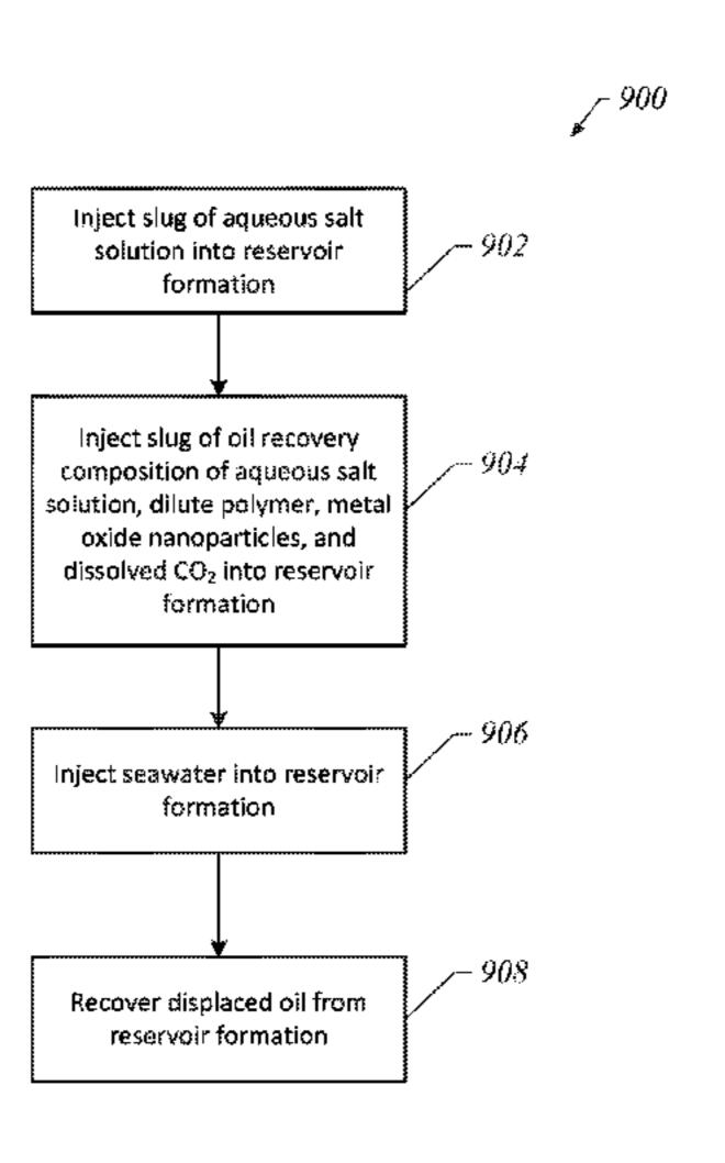
compositions provided may be suited for enhancing oil recovery in carbonate reservoirs having in situ oil viscosities less than 3 centipoise (cP).
