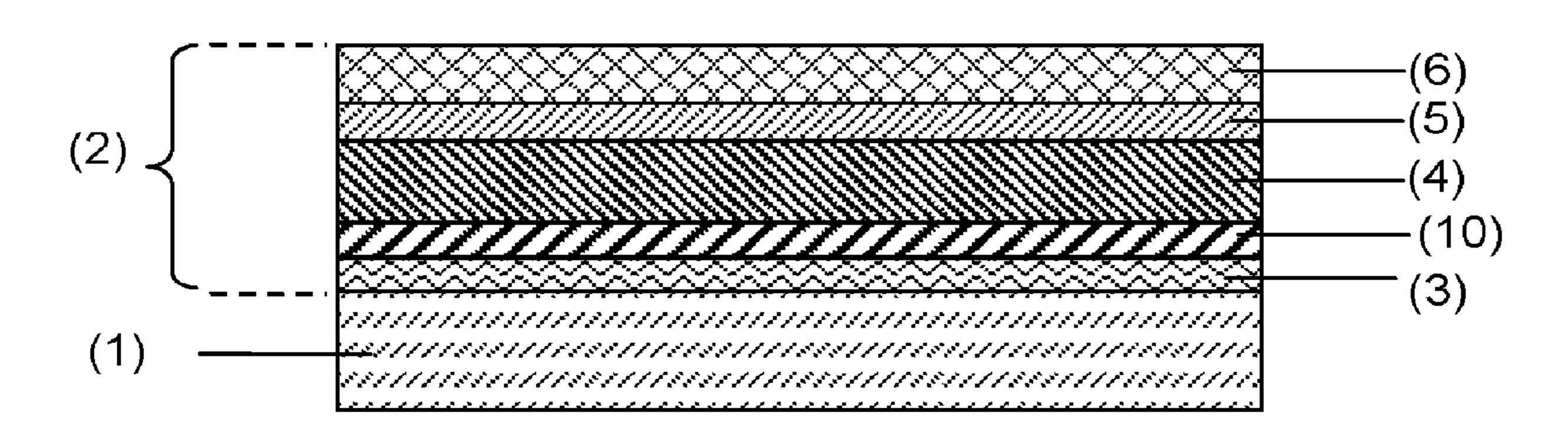
and wherein the darkening layer (10) contains at least one metal, one metal nitride, and/or one metal carbide with a melting point greater than 1900° C. and a specific electrical resistivity less than 500 μohm\*cm.
