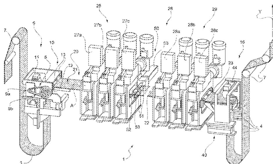
second distance along direction; feeding group comprises: advancing device controllable to arrest web in a position, at which second area is spaced an intentional offset from second desired position; and an actuator controllable for moving second area towards second desired position to recover offset; absolute value of difference between first and distances being equal to offset.
